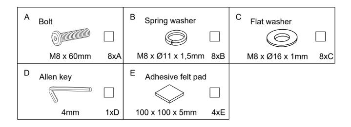
Step 1: Using two people carefully turn the table top (1) upside down. Attach table top (1) and legs (3) as shown in diagram using bolts (A) and washers (B&C). Tighten using the allen key (D) provided, then attach adhesive felt pad (E) onto the legs.
